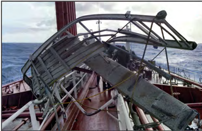
"Stolt Surf" – one of the gangways curled up on the catwalk (Photography by Karsten Petersen ©)
